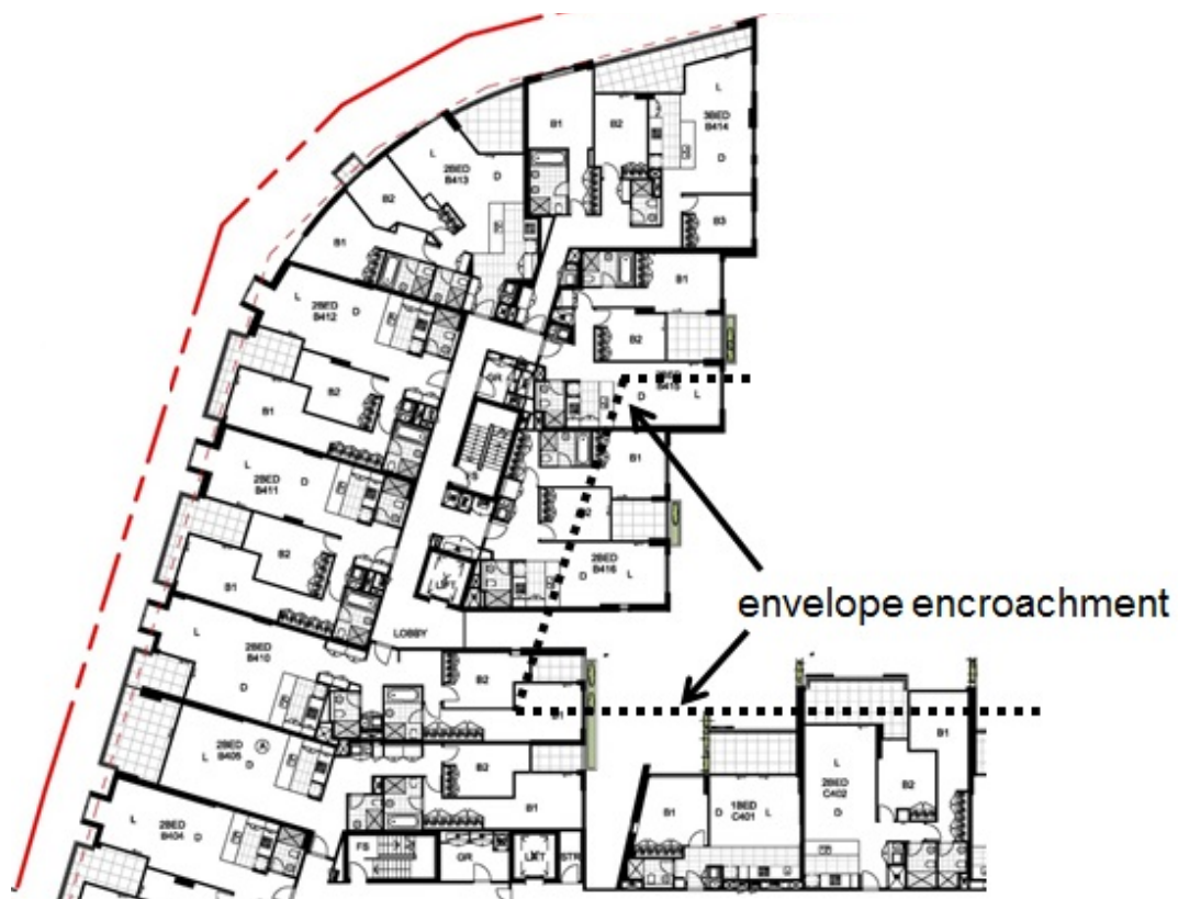
Figure 19: Stage 1 encroachment Building 5B Levels 1-5
